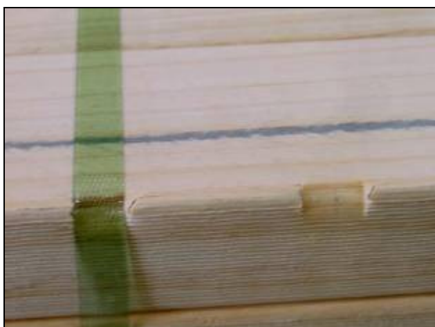
Pic. 7 Corner damage PET / Steel Strap comp
