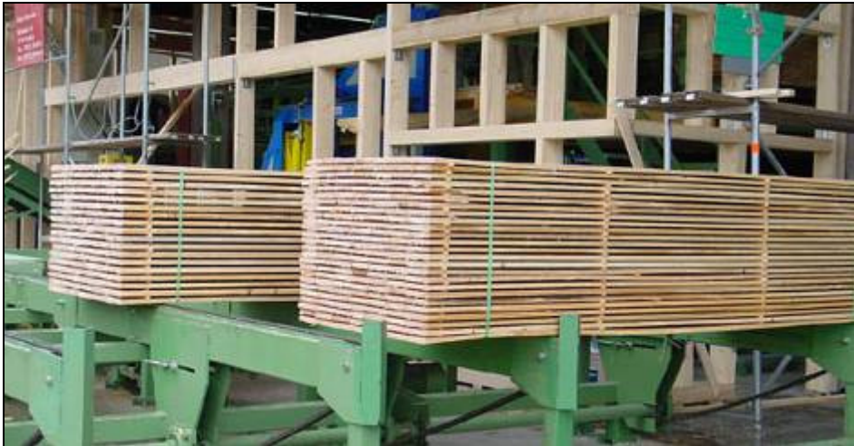
Pic. 9 Green wood packs with fillets
