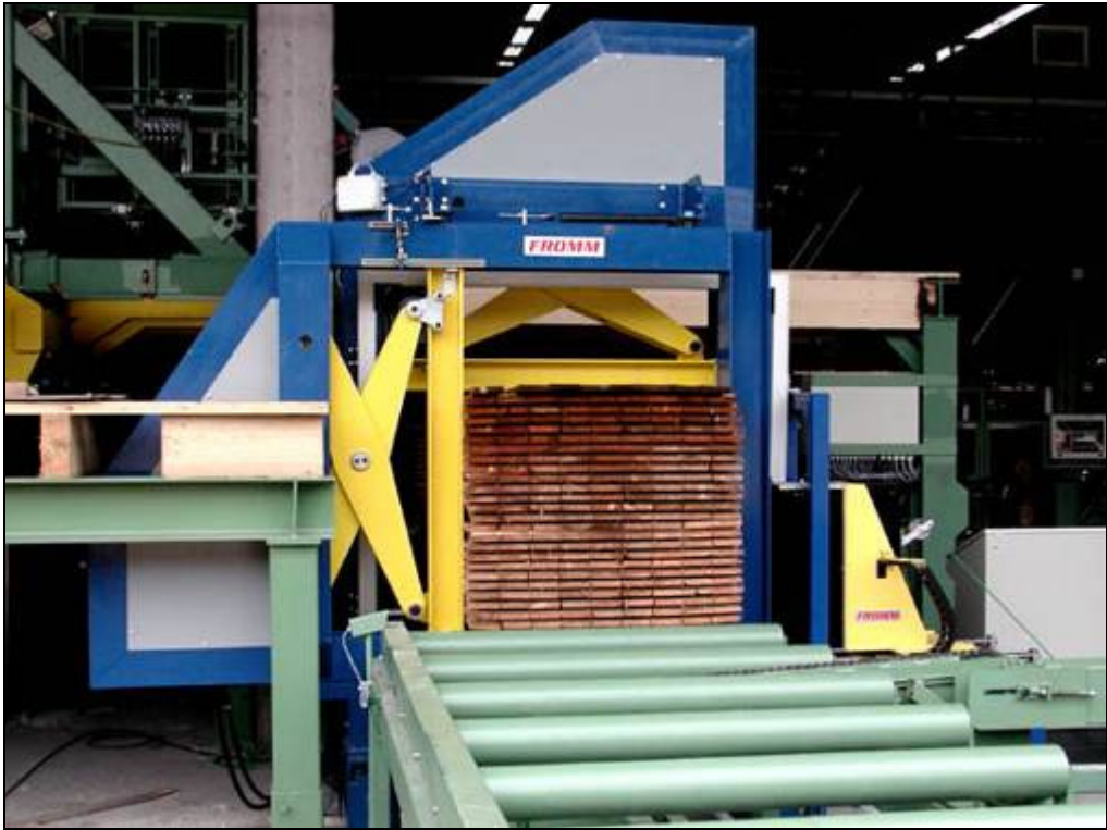
Pic.10 Fully automatic lumber strapping press
