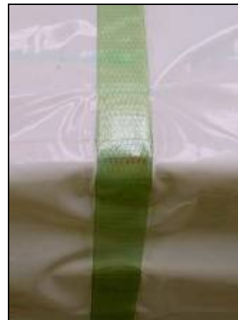
Pic. 6 Min. corner damage by PET
