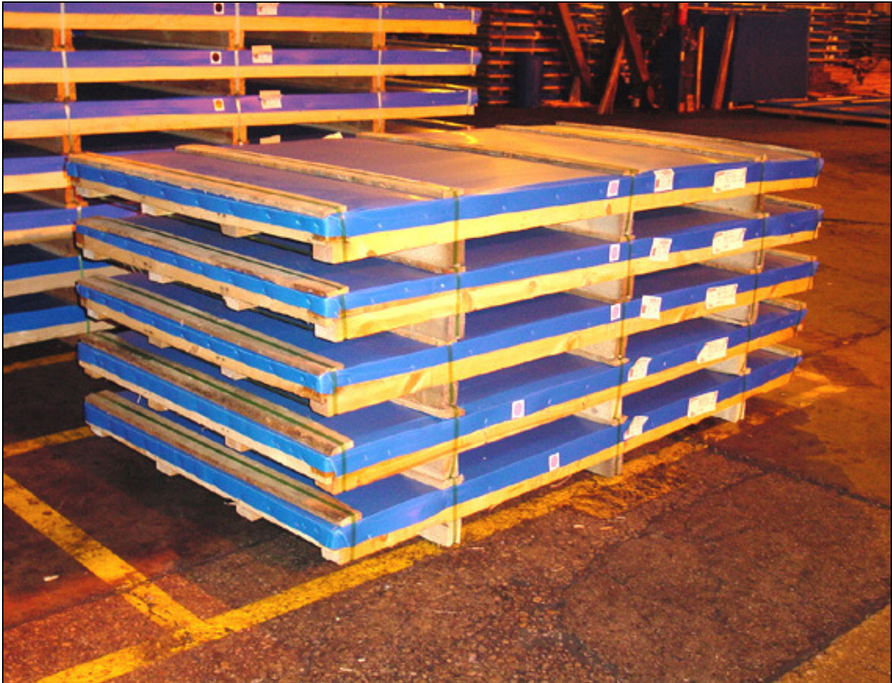
Pack covered with plastic corrugate board, stapled and top cross board strap down with PET
