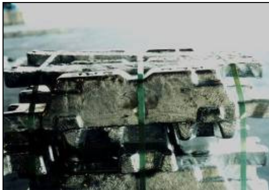
Pic. 4 Top stabilizing during strapping required
