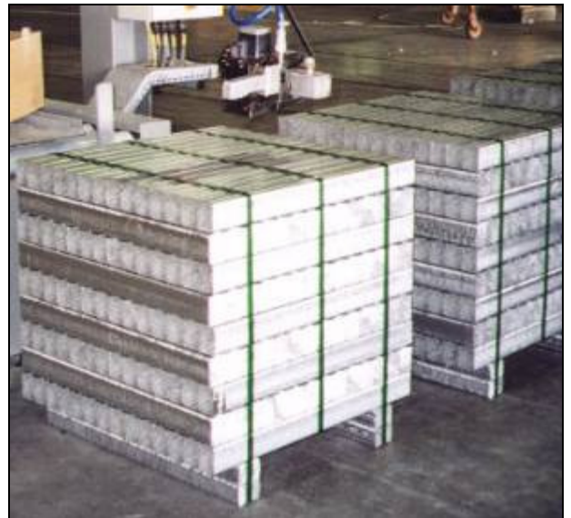
Pic. 5 Horizontal extruder ingot bar, cut and stacked and strapped
