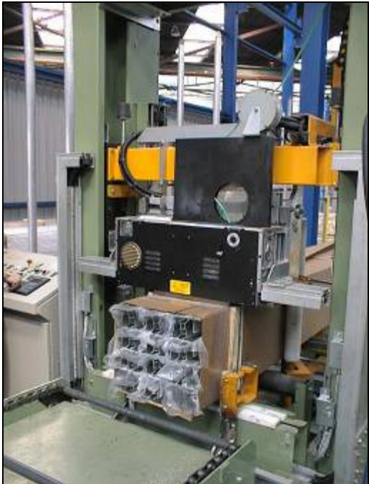
Pic. 8 Manual applying boards but automatic strapping
