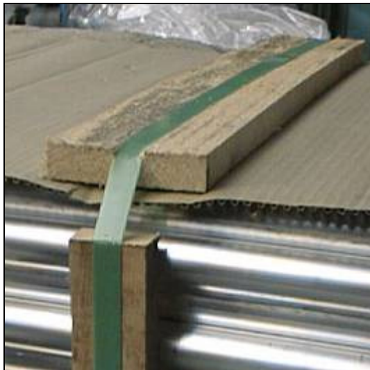
Pic. 5 Strapping detail
