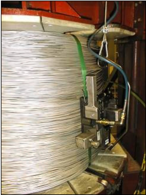
Pic. 4 PET strapping on press
