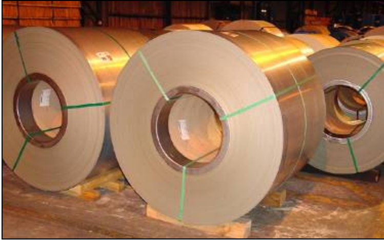
Pic. 2 New package securing with PET strap
