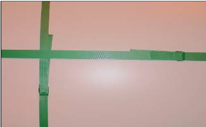
Pic. 4 PET Seals. Strapping around the diameter is limited. Min. coil OD is 1000mm (39"). Tension loss by the tool and splitting danger in seal area.
