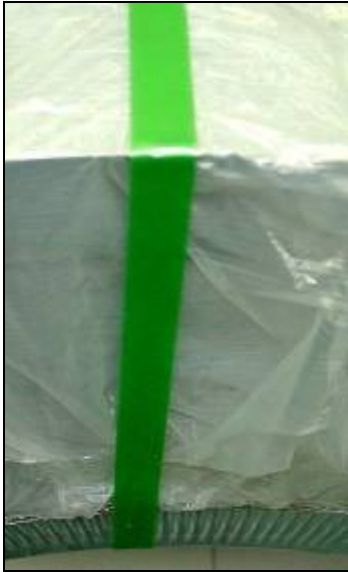
Pic. 5 Sharp edges do not cut PET strap
