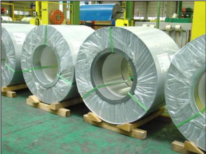
Pic. 3 Coils additionally wrapped with plastic.
