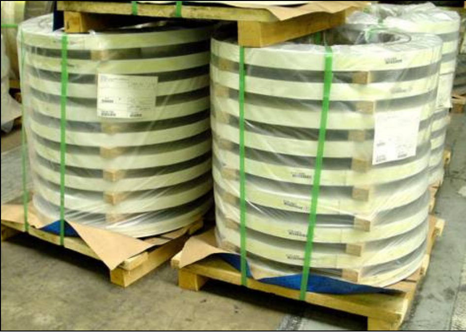
Pic. 4 Coils strapped down through the eye
