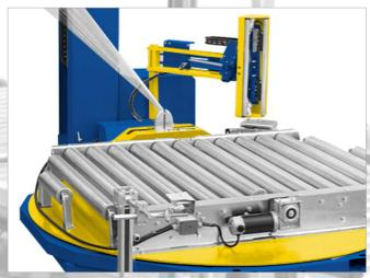
Incorporating all belonging functions of attaching, clamping, cutting and wiping the film end to the package.
